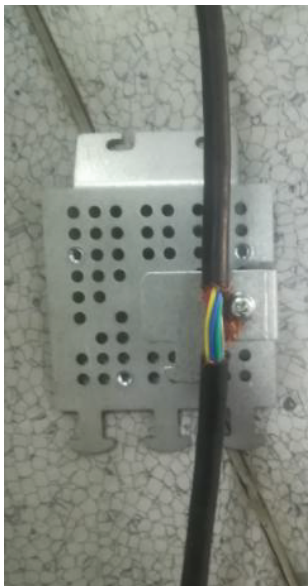
EMC wiring of Power Module B1
