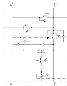
图6 马达集成阀块 Figure 6 motor integrated valve
