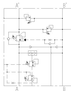
图7 马达集成阀块 Figure 7 motor integrated valve
